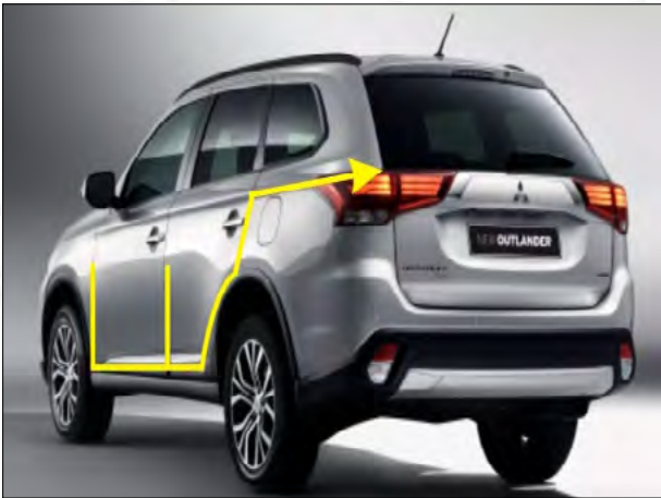
11. The power cable and the central control cable follow the yellow arrow through the rubber plug until the tailgate cover.
